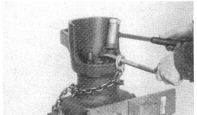
Fig. 286—Use a chain and pry bar to apply downward force on bevel pinion shaft and strike end of shaft several times with a soft hammer to seat pinion bearings.
